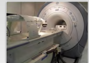
Innomotion MRI-compatible robotic arm (Innomedic GmbH) and 1.5T GE MRI scanner at IMSaT
